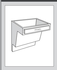
Universal Design Base Cabinets are 321/2" high by 20  $\ensuremath{\ensuremath{\mathcal{Y}}}\xspace''$  or 24" deep. The toe kick is 8" high and 61/2" deep to accommodate most wheelchair footrests.
