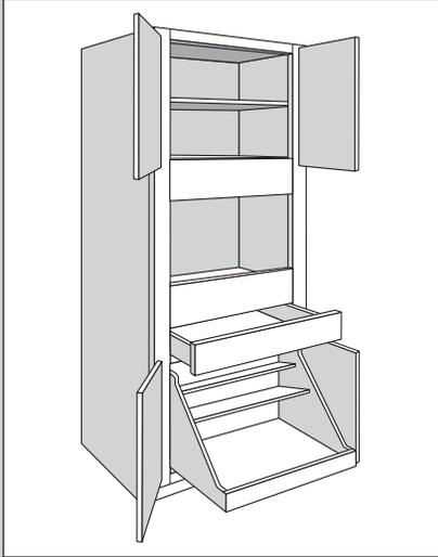
Oven cabinets range in size from 27" to 33" wide, from 84" to 96" high and are 24" deep.
